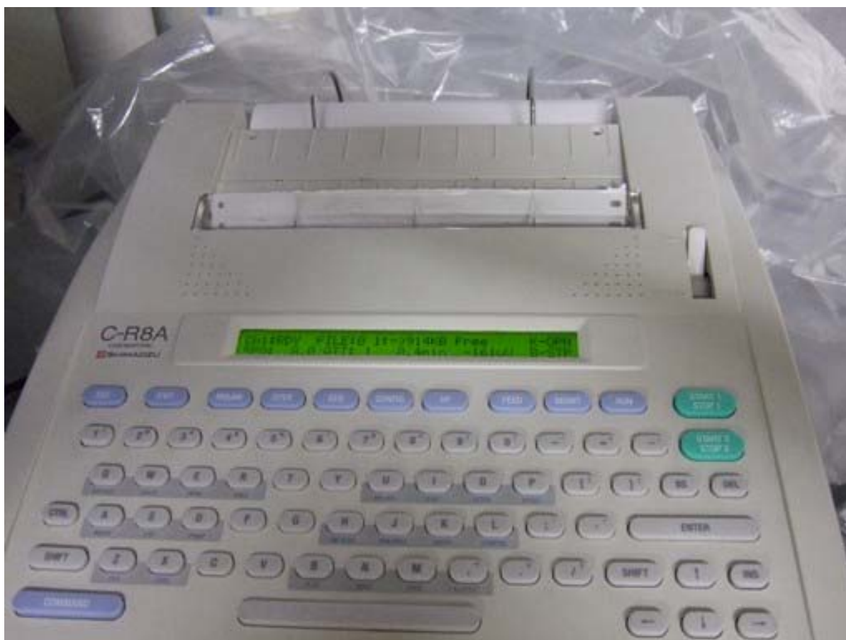
Figure 18. This is a standard integration apparatus supplied from Shimadzu (C-R8A). It is not only useful for the manual injection routines but also useful for the automatic measurement routines, since it can run under a Basic program, which can be used for starting or stopping the analysis by the talking through a serial port. The results of data can also be transferred from the C-R8A to the PC by the talk through the serial port. KS is now planning to adapt this integrator for the new automatic system under construction.
