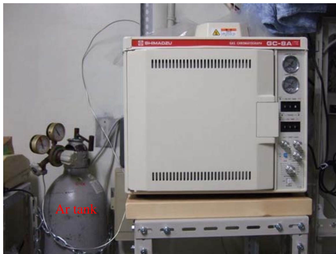
Figure 16. A Shimadzu GC-8AIT, which is used for the manual method. It gives a slightly different response upon the change in pressure when a relatively large volume of gas was injected. In case of GC-14A used in the automatic measurement system, a large shift is given with regard to the base line so that the calibration of the peak area has some difficulties in the case of our previous GC-14A system. We are now planning to adopt this GC for developing our new automatic hydrogen measuring system in the near future.
