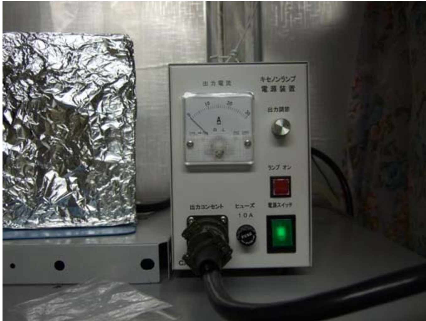
Figure 19. The electrical power supplier for the new Xe lamp: a ILC Technology CERMAX LX-300 Xe lamp equipped with a CM-2 cold mirror ( 240 < \lambda < 550 nm), operated at 300 W. This is a very good Xe lamp whose cost is also reasonable.
