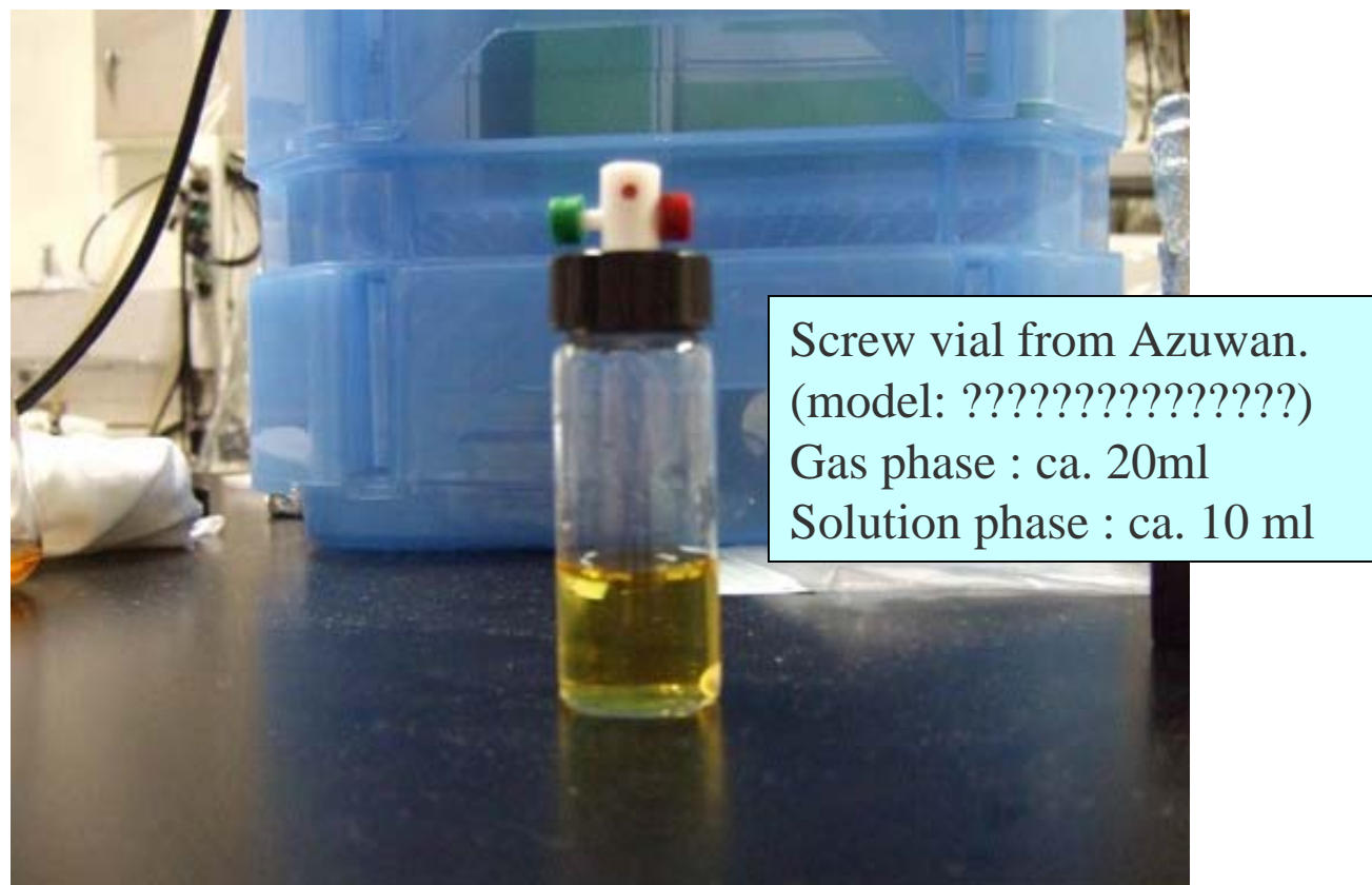
Figure 17. The special screw vial possesses a teflon gas collection unit, equipped with a teflon valve which can be manually opened or closed for the gas collection using a gas tight syringe. For the complete substitution of the gas inside the vial, we use a plastic bag in which the vial involving solution and a stirring chip, together with a cap equipped with the septum unit, is sealed located inside the bag, and the solution was bubble with Ar for at least 30 min, during which the gas phase inside the bag is also purged and substituted well with Ar. Finally, the cap of the vial was closed inside the sufficient flow of Ar without having the leak of air into the vial.
